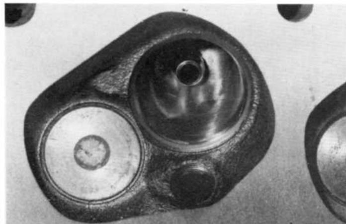
Finished port with aluminium/Bronze guide insert. Guide does not restrict flow with the right shaped port.
