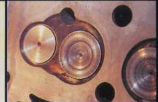
The early (681F) crossflow 1.6 engines had shallow combustion chambers in the head and the rest were in the piston crown. The 1.1 and 1.3 units had flat heads.
