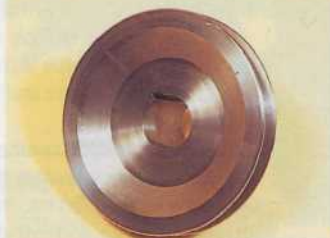
Ideally a steel front pulley needs to be fitted to the high revving Crossflows as the stock item is a lot weaker and can shatter.
