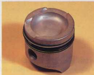
Stock crossflow pistons (above) are suitable for up to 7000 rpm. Beyond that forged Accralite items (below) are the best bet.
