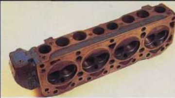
This pre-crossflow cylinder head shows both inlet and exhaust ports on one side and has full-size combustion chambers.
