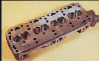
Late (711M) crossflows had totally flat cylinder heads and combustion chambers in the piston crown.
