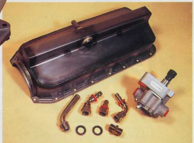
Fitting a dry sump kit will eliminate oil surge and improve flow in competition engines. A remote oil tank will also need to be fitted.
