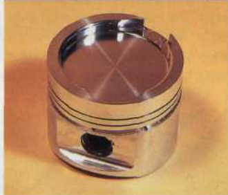
Stock crossflow pistons (above) are suitable for up to 7000 rpm. Beyond that forged Accralite items (below) are the best bet.
